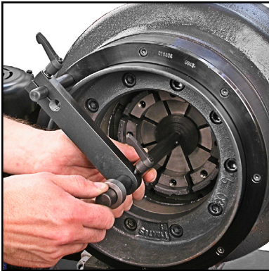
Loosen the Coupling Stop Clamp and position the Coupling Stop against the back face of the dies.
